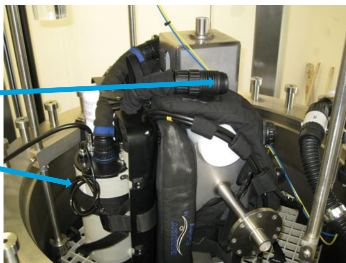
Inspiration rebreather in place ready to start test
