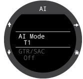
When **AI Mode** is set to **Off**, the AI sub-system is completely powered down and does not consume any power. When on, the AI system increases power consumption by approximately 10%.
