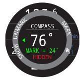
From this pop-up you can mark and unmark headings and show or hide the Outer Ring compass overlay.
