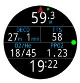
When the overlay is enabled, green arrows at the top of the display indicate the direction of your mark when more than 5 degrees off course.
