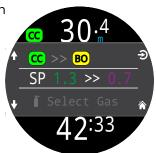
Pressing SELECT when this menu item is displayed changes the PPO2 set point from the low set point to the high set point or vice-versa. To redefine the PPO2 value of a set point, use Main Menu > Set points.
