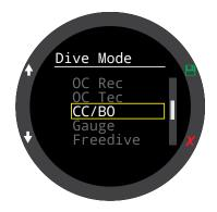
When changing to or from Gauge or Freedive Mode, the decompression tissues are cleared. This is because when in these modes the Teric does not know what gas you are breathing, and therefore cannot track inert gas loading. Plan repetitive dives accordingly.
