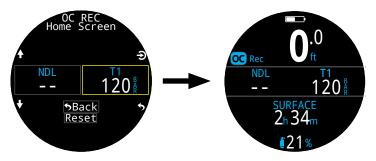
In any SCUBA mode, when using the Standard layout, the info row can be customized extensively to show AI information.
