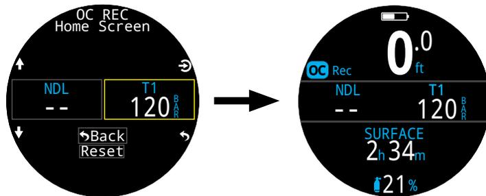
In any SCUBA mode, when using the Standard layout, the info row can be customized extensively to show AI information.
