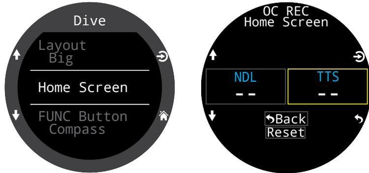
The Big layout (default for OC Rec mode) allows for customization of the right info row slot only because the left slot is taken by NDL which cannot be permanently obscured.
