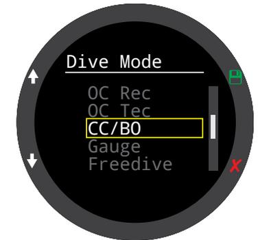
When changing to or from Gauge or Freedive Mode, the decompression tissues are cleared. This is because when in these modes the Teric does not know what gas you are breathing, and therefore cannot track inert gas loading. Plan repetitive dives accordingly.
