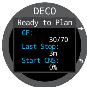
When the correct values are entered, select "Run Plan" and confirm decompression settings and starting CNS.
