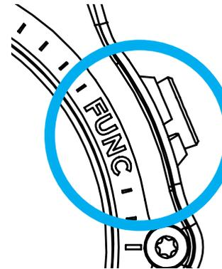
The function (upper right) button is a customizable shortcut that makes accessing your most used functions on the Teric a little easier.
