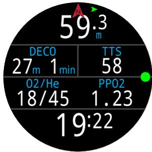
When the overlay is enabled, green arrows at the top of the display indicate the direction of your mark when more than 5 degrees off course.
