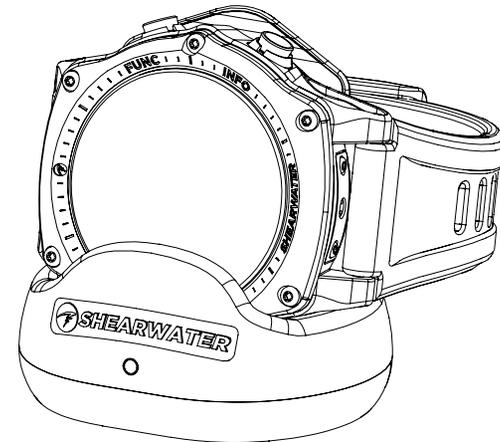
The Teric screen rotates 90 degrees for easy viewing of the time when the Teric is mounted on the charger.
