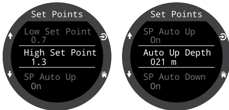
If **SP Auto Up** is set to "On", use **Auto Up Depth** to set the depth at which the auto switch occurs.
