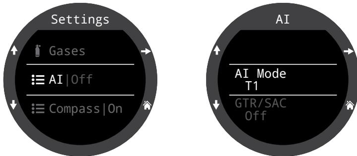
When **AI Mode** is set to **Off**, the AI sub-system is completely powered down and does not consume any power. When on, the AI system increases power consumption by approximately 10%.
