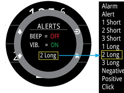
Use the up and down arrows to select an alert and press select to test it.
