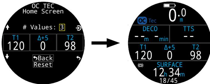
In the Open Circuit Rec mode, the right slot of the center row is also customizable.
