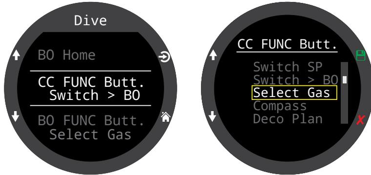
In CC/BO mode there is a separate function button shortcut for each CC and BO. This allows you to optimize computer's operation in advance, minimizing button pushes during an emergency.
