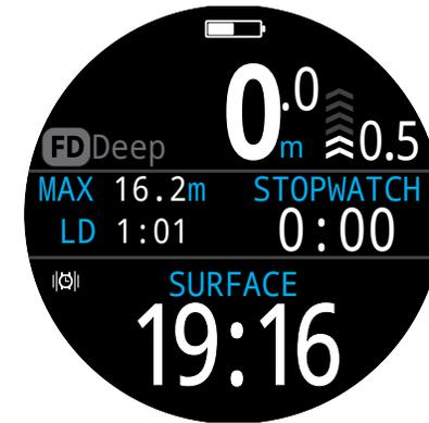
Like in OC Rec and Gauge Mode, in Freedive Mode, the right home screen slot can be customized in the Big Layout.
