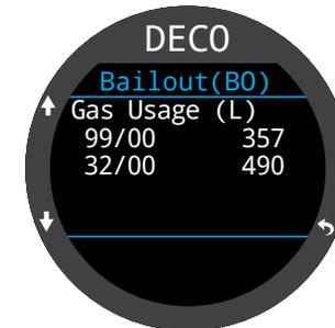
If no decompression is required, no table will be shown. Instead, the total No-Decompression-Limit (NDL) time in minutes, at the given maximum depth will be reported. Also, the gas quantity required to surface (bailout in CC) will be reported.
