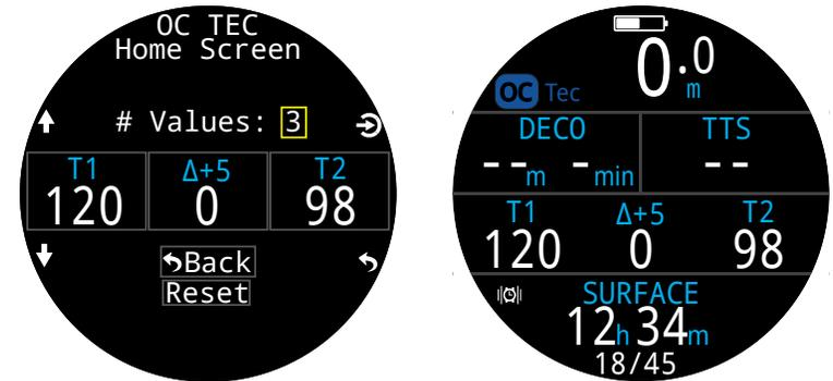
In CC/BO mode there is a separate Home screen menu item for each CC and BO. This allows you to optimize your bailout screen layout in advance, minimizing button pushes during an emergency.
