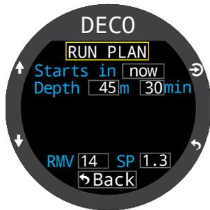
Enter the expected surface interval, bottom depth, bottom time, respiratory minute volume (RMV) and Set Point (closed-circuit only).
