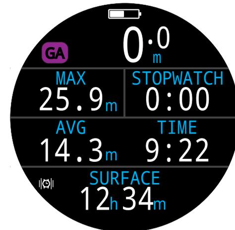
*Standard layout - Alternate Gauge Mode configuration.*
