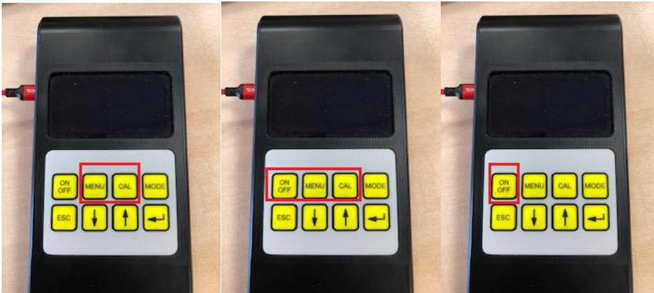
11. Once the analyzer is in the Bootloader mode (screen will remain blank) and the ON/OFF is continually pressed you will select in FLIP program RS232 window > **Connect**. The RS232 window will collapse. Continue to hold ON/OFF button.
