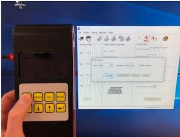
12. On the now available page press RUN button in lower left corner and let the FLIP program install the new FW. This process can take a while, please be patient and make sure you do not release the ON/OFF button. If you do so, you'll need to restart the whole process and begin at point #1.
