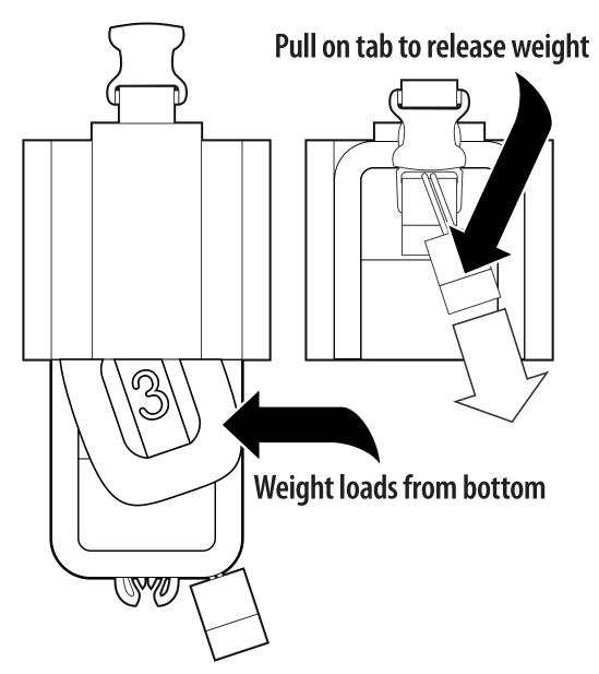
Figure 3b: Weight system operation
