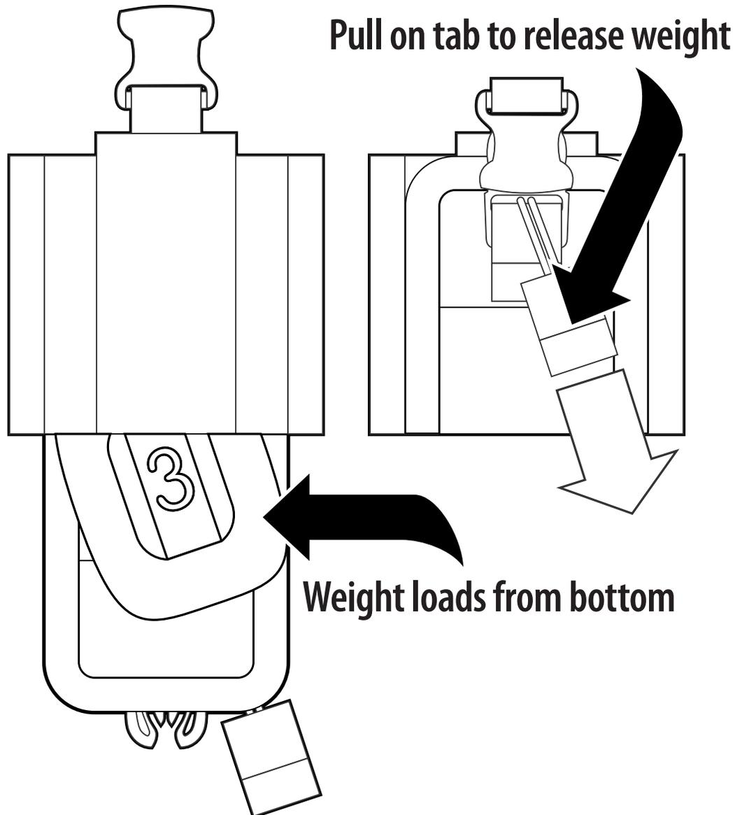
Figure 3b: Weight system operation
