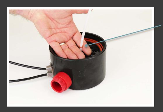
The oring should be above the sensor disk. To ensure its in the right spot lay your fingers on the disk and the oring should be above your fingers. When the canister is installed it will push the oring down to seal against the s/s rod in the center of the canister.
