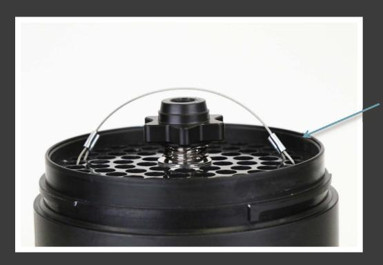
When packing with granular, fill and tap to ensure its tight. Fill to ¼ inch from the top and place the top plate on the canister and it should be flush with the inside edge of the canister. Use the nut and spring to hold tension on the top plate. Do not use the nut and spring to apply pressure to pack the scrubber. The spring and nut are to ensure an even pressure is held on the top plate after properly packing it.
