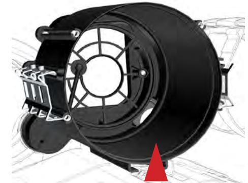
Figure 1-66. Inspect and lubricate cartridge housing end cap radial sealing surface.
