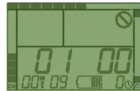
Figure 2-3. When the top and bottom segments on the display starts to blink, re-connect the wet-switches.
