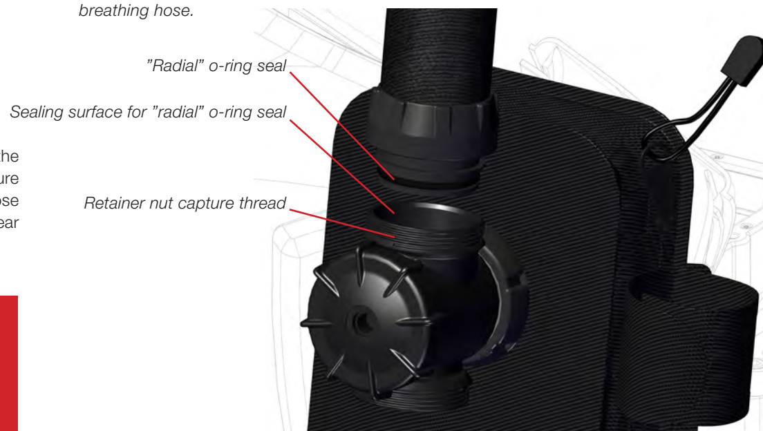
Figure 1-32. Attach the left rear breathing hose to the left counterlung shoulder port.
