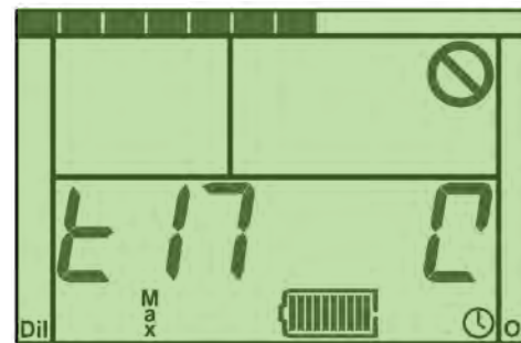
Figure 2-5. Test 17 (Backlight Power consumption), displaying test number on the left and the “spinning wheel” on the right.
