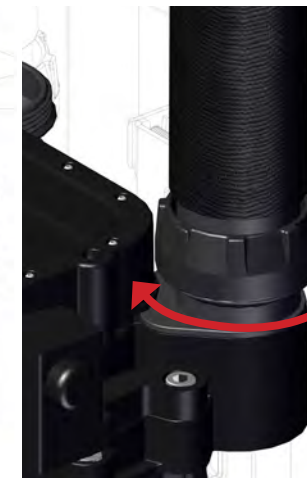
Figure 1-30. Hand tighten the swivel capture nut: Do NOT use tools or over-tighten.
