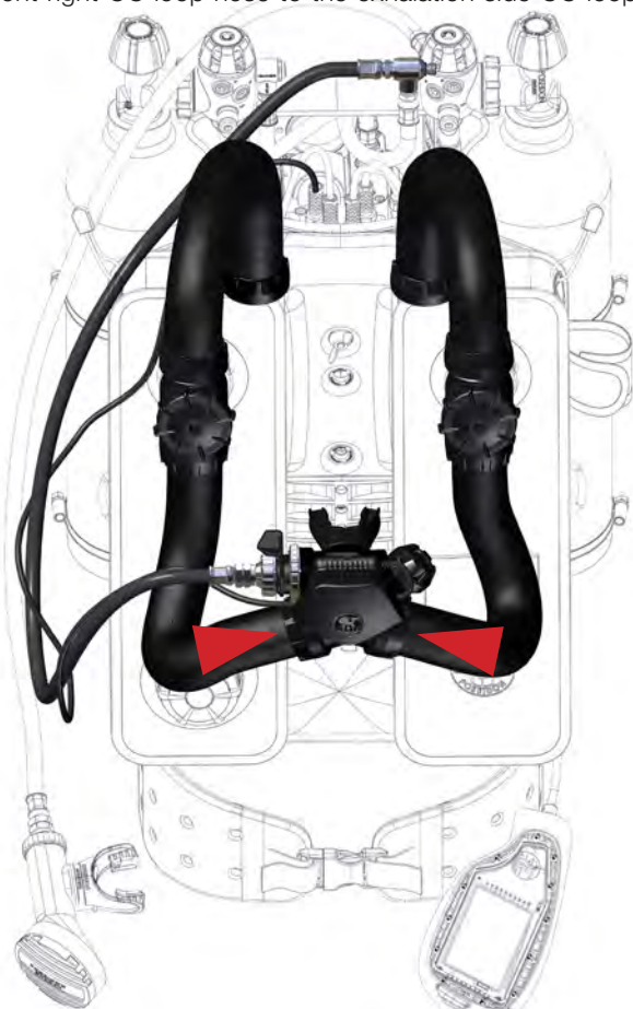
Figure 1-49. Breathing hoses properly connected to the mouthpiece.
