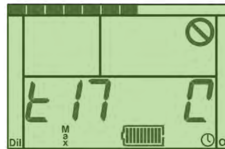
Figure A1-1: Test 17 (Backlight Power consumption), displaying test number on the left and the “spinning wheel” on the right.
