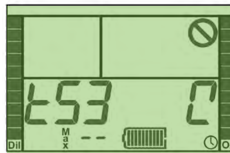
Figure 2-11. Test 53 – Oxygen Sensor calibration.
