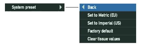
This is a quick way to configure the unit to be used in Metric (EU) or Imperial (US) mode. This will only affect the metric and imperial part of the settings. Use the "Factory default" to reset the settings back to factory settings. This will not erase any dive log, redbox log or any pictures, only set the settings back to default.
