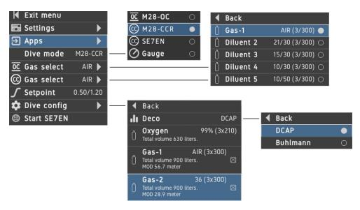
In M28 Closed Circuit mode the M28 will guess the gas mixture that the diver is breathing based on the settings selected. If a CPOD with an oxygen sensor is connected and mounted on the loop the decompression model will use this as input.
