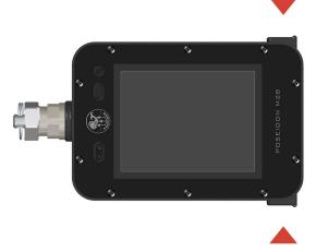
Once the M28 has been started, the green indicator light will flash to indicate that the M28 computer is turning on. This will be followed by a start-up screen with a visible Poseidon logo. Please note that the time to visible start-up screen can vary in length. After a few seconds this screen will be replaced by the land app, recognized by a large central analogue clock.
