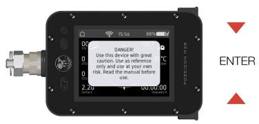
On the following pages the various application modes will be discussed, as well as the menu structure. The "Land" app is the initial app after start up. This app is automatically visible after an initial safety message that can be confirmed by pressing either one of the two buttons.
