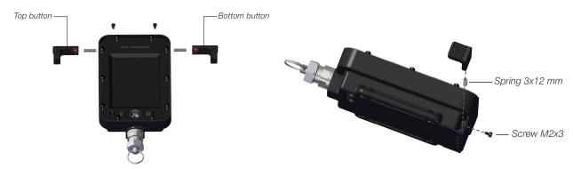
Make sure to re-install the compression spring correctly and the buttons are placed on the correct side because these are different. Hand tighten the screws carefully. Buttons, springs and screws are available to be ordered as spare parts. When assembling new buttons those shall be recalibrated through the PC software.
