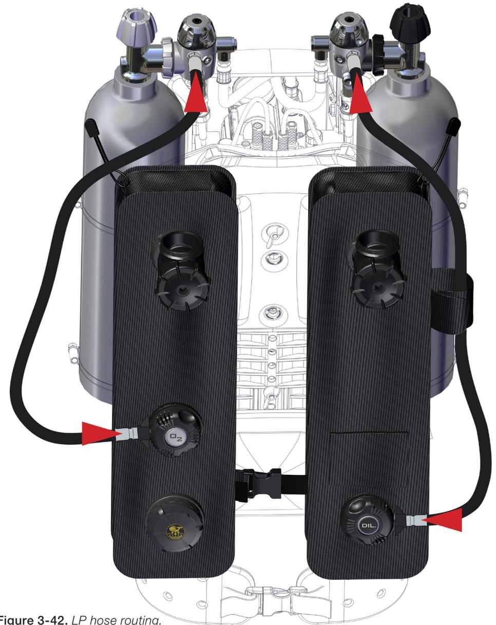
Figure 3-42. LP hose routing.
