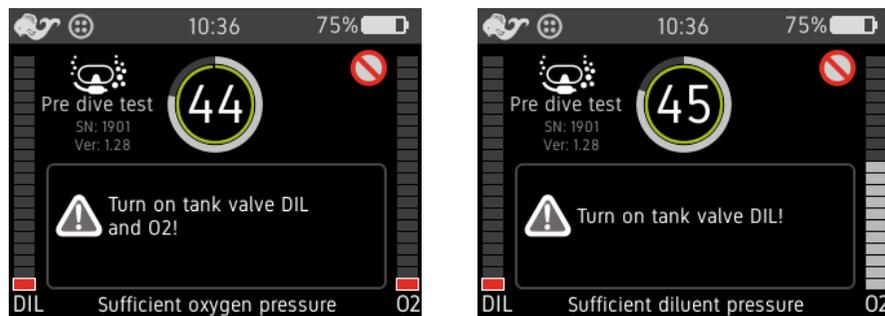
Figure 2-8. Tests 44 and 45, confirming sufficient gas supply pressures.
