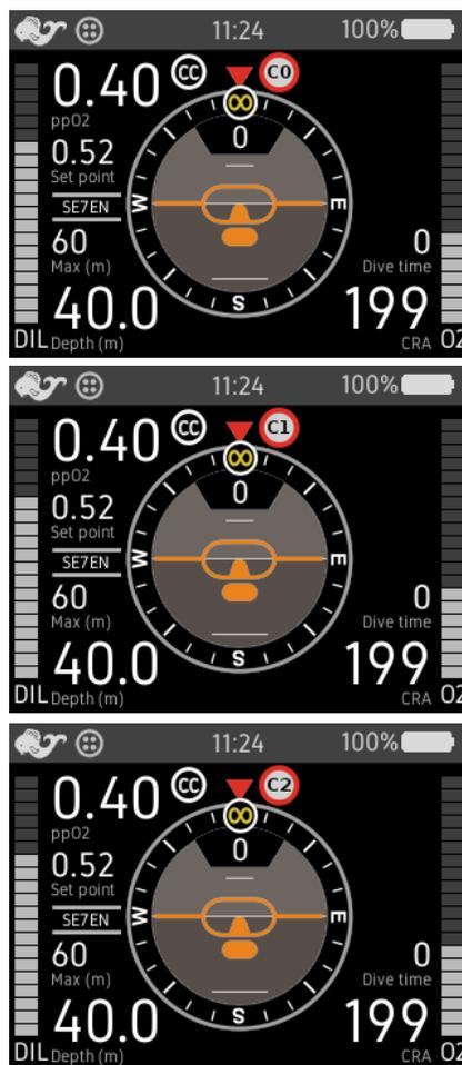
Figure 3-16. Oxygen sensor confidence alerts: C0, C1, C2.
