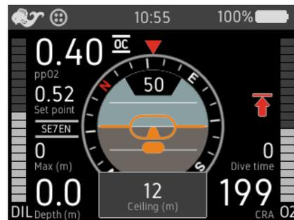
Figure 3-11. Decompression ceiling alert.
