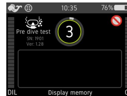
**Figure 2-3.** PreDiveTest display where the number in the circle represents the test number together with an explanatory text at the bottom of the screen.
