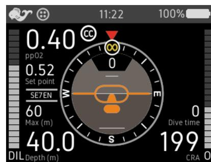
Figure 3-17. Closed Circuit mode.
