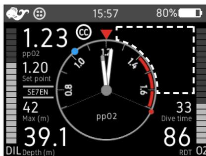
Figure 3-6. Alarm signal area.
