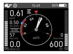
**Figure 2-14.** *Ready-to-dive. At this point,the pre-dive tests are completed, and the system is ready to dive.*
