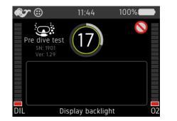
Figure 2-5. Test 17 (Backlight Power
