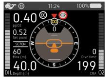
Figure 3-16. Oxygen sensor confidence alerts: C0, C1, C2.
