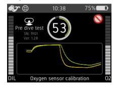
**Figure 2-11.** *Test 53 – Oxygen Sensor calibration.*
