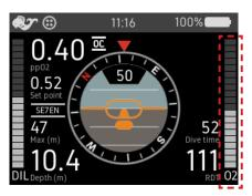
**Figure 3-32.** Oxygen cylinder pressure indicator.
