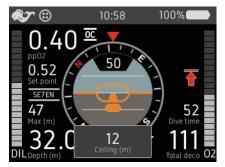
**Figure 3-23.** *Display indicating "ceiling" to which it is safe to ascend & total decompression time.*
