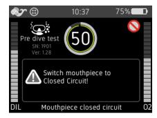
**Figure 2-10.** *Test 50 – Closed-Circuit mouthpiece position.*
