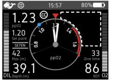
Figure 3-6. Alarm signal area.
