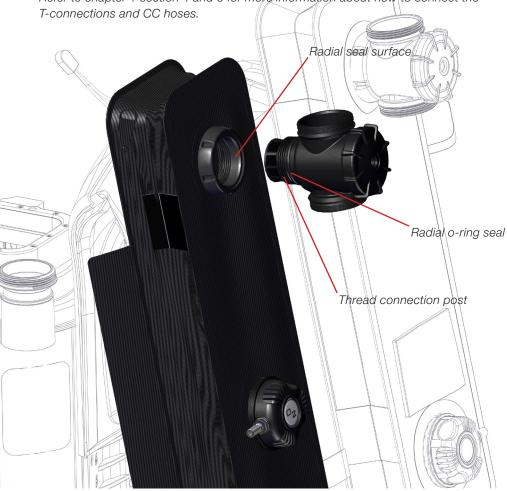
**Figure 3-40.** Insert the right hand water diversion manifold into the port on the right counterlung. Clockwise tighten the water diversion manifold into the right and left counterlung shoulder port. Note the correct orientation, further described in chapter 1, section 4.
