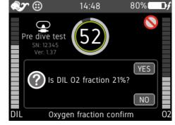
**Figure 3-44:** Oxygen confirmation screen at test 52, showing the question of oxygen fraction content in the diluent gas tank.
