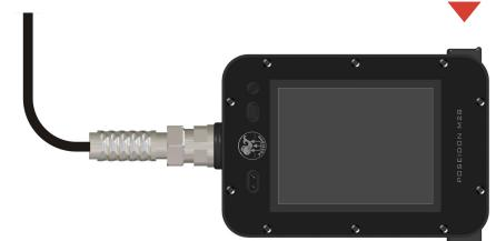
**Figure 2-1.** *Press both buttons simultaneously for power up.*
