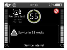
**Figure 2-12.** Test 55 – Service interval check.
