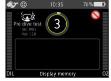
**Figure 2-3.** *PreDiveTest display where the number in the circle represents the test number together with an explainatory text at the bottom of the screen.*
