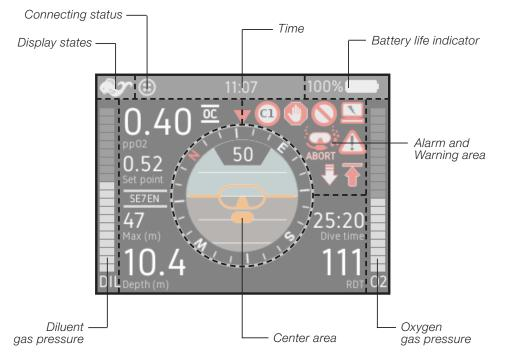
Figure 3-2. LCD display layout.
