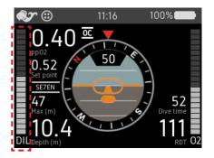
**Figure 3-31.** Diluent cylinder pressure indicator.
