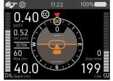
Figure 3-17. Closed Circuit mode.
