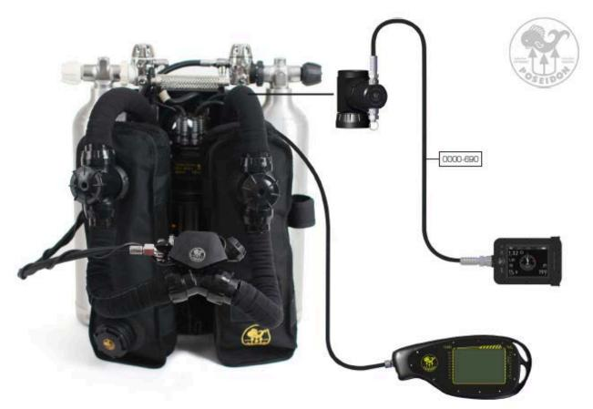
**Tec Spec 1:** The M28 uses a single cable (0000-690) to connect to the C-POD, using either a galvanic or a solid state as a third cell. The SE7EN uses the paddle display. This configuration is also suitable for a Poseidon MKVI.
