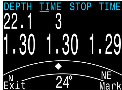
The marked heading is shown with a green arrow. When within 35° of the heading, the degrees display turns green.
