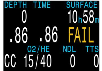
**All sensors display FAIL after calibration**
