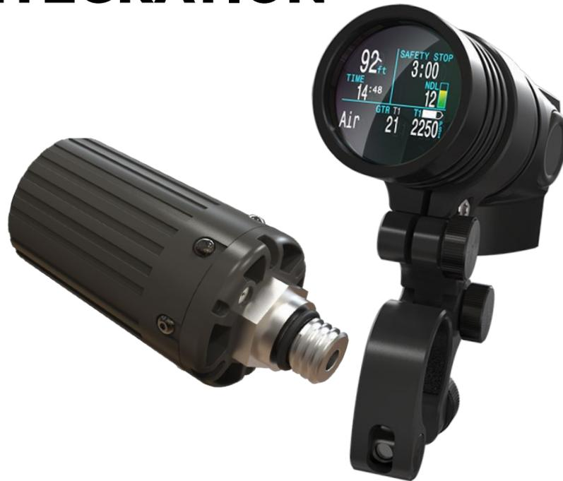
All NERD 2 models are equipped with dual transmitter air integration capability. For complete information on how to operate the various features of AI, see the [PERDIX AI Operating Instructions manual](#).
