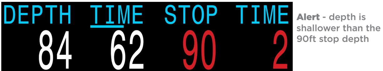
By default the NERD 2 uses a 10ft (3m) last stop depth. At this setting, you may perform the last stop at 20ft (6m) with no penalty. The only difference is that the predicted time-to-surface will be shorter than the actual TTS since off-gassing is occurring slower than expected.
