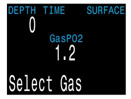
Use the MENU button to increment to the desired diluent/gas, then press the SELECT button to select that diluent/gas.
