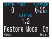
Restore mode can be toggled on and off. When toggled on, it shows deleted logs, greyed out in the "Display Log" sub-menu. These dives can be restored to the Dive Log.
