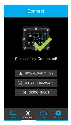
The NERD 2 screen will give percentile updates while receiving the firmware, and the phone will read "Firmware successfully sent to the computer" upon completion.
