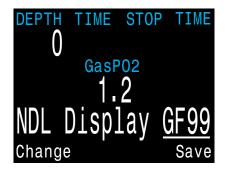
15 **GF99**  The number shown is the percentage of supersaturation. The number is calculated by reference to the Ambient Pressure Line and the
