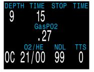
When we clear the last stop, the stop depth and time goes blank, and now we see a NDL of 99 minutes again. Once we surface, the depth is 0 and a minute later when the computer comes out of dive mode, the NDL goes to 0 as well.
