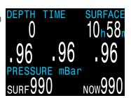
The 0.96 PPO2 result is, in this case, correct. At high altitudes, the difference between FO2 and PPO2 will be even larger. To see the current pressure, start at the main screen and press the SELECT button a few times (displays as Pressure mBar NOW).
