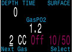
A gas that is off will be shown in **Magenta**, but can still be selected. It will be turned on automatically if it is selected. Off gasses are not used in decompression calculations.
