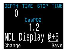
The next selection is @+5. This feature was inspired by Dan Wible's CCR2000 computer (Thanks Dan!). It is the time-to-surface (TTS) if you were to stay at the current depth for five more minutes. This can be used as a measure of how much you are on-gassing or off-gassing.
