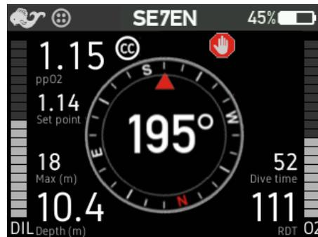
The Stop alert symbol located in the Alarm Signal Area, is displayed if the diver is ascending too rapidly. The appropriate response is to immediately stop ascending, and the diver should maintain the current depth until the symbol disappears.
