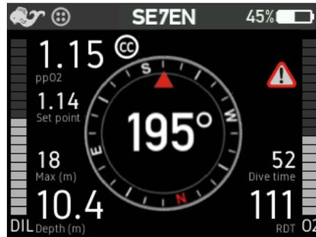
The General alert symbol located in the Alarm Signal Area will flash in synchrony with any other parameter(s) on the screen that is/are inappropriate or out of acceptable range. This signal is intended to catch the diver's attention, and prompt the diver to scan the other elements on the screen to see which value(s) is/are also flashing. As long as one of the other displayed values on the Primary Display is flashing, the General Alert symbol will also flash.
