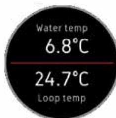
**Temperature.** Displays the current water temperature when you dive. If SE7EN is connected also displays the temperature in your breathing loop. The unit (°C or °F) can be configured in Settings / Temperature unit.
