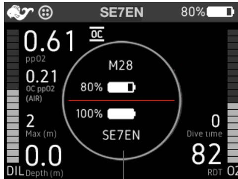
*Battery status can be displayed in the Center area for multiple devices simultaneously.*
