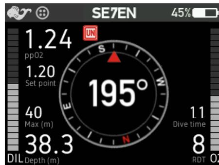
Directly to the right of the PO2 value the mouthpiece position is communicated:
