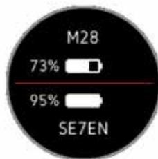
**Battery status.** Displays the battery status (% of capacity when the battery is fully charged). If a SE7EN is connected, the M28 also displays the SE7EN battery status. The battery icon in the Top Bar always shows the battery status for the M28.
