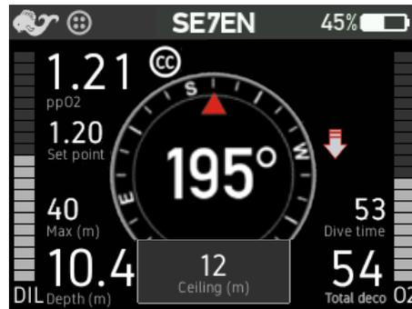
In the unlikely event that a diver incurs a decompression obligation (i.e., the Decompression Ceiling Alert is displayed), and the diver then ascends above the depth at which the Decompression Stop Alert is displayed, the Descend arrow will flash. In this situation, simply descend gradually until the Descend arrow no longer flashes, and remain at that depth until the Decompression Stop Alert no longer displays.
