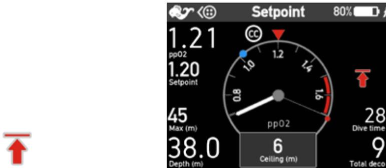
The Decompression ceiling alert symbol will flash when the diver has incurred a decompression obligation. The current decompression stop is displayed in a text message.
