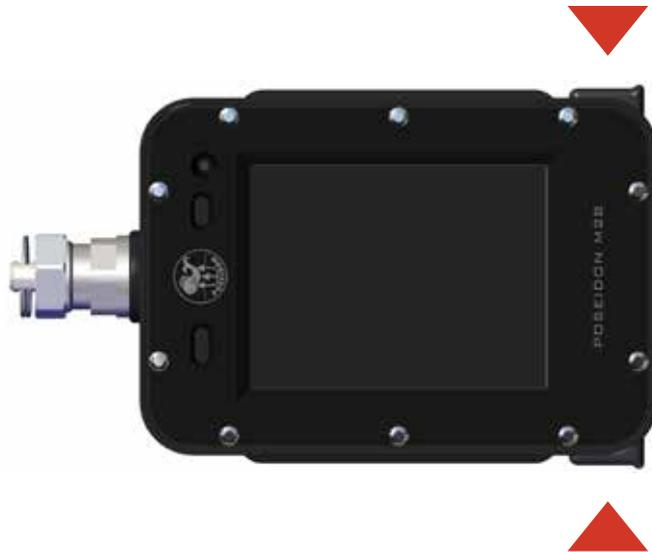
Once the M28 has been started, the indicator light will flash green to indicate that the M28 computer is turning on. This will be followed by a start-up screen with a visible Poseidon logo. Please note that the time to visible start-up screen can vary in length. After a few seconds this screen will be replaced by the Dive app.
