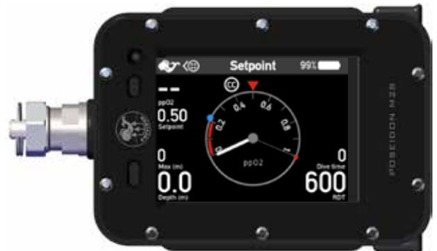
On the following pages the various application modes will be discussed, as well as the menu structure. The “Dive” app is the initial app after start up. This app is automatically visible after an initial safety message that can be confirmed by pressing any of the two buttons.
