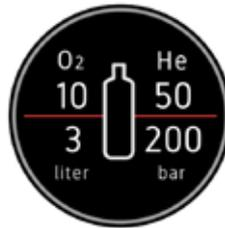
**Cylinder pressure and gas.** Displays the configuration of the currently selected gas tank in terms of tank volume, tank pressure rating, oxygen fraction and helium fraction. This center view is automatically selected when switching gases, changing from closed circuit (CC) mode to open circuit (OC) mode on SE7EN or when activating bailout in Setpoint mode.
