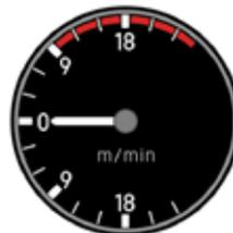
**Ascent/Descent rate.** Shows Ascent and Descent rate per minute. Unit (m/min or ft/min) is configured in Settings / Depth unit. Ascent rate alarm will start when Ascent speed is higher than 9 meters/minute. There is no descent rate alarm, but remember that ppO<sub>2</sub> in the gas will change when depth is changing.
