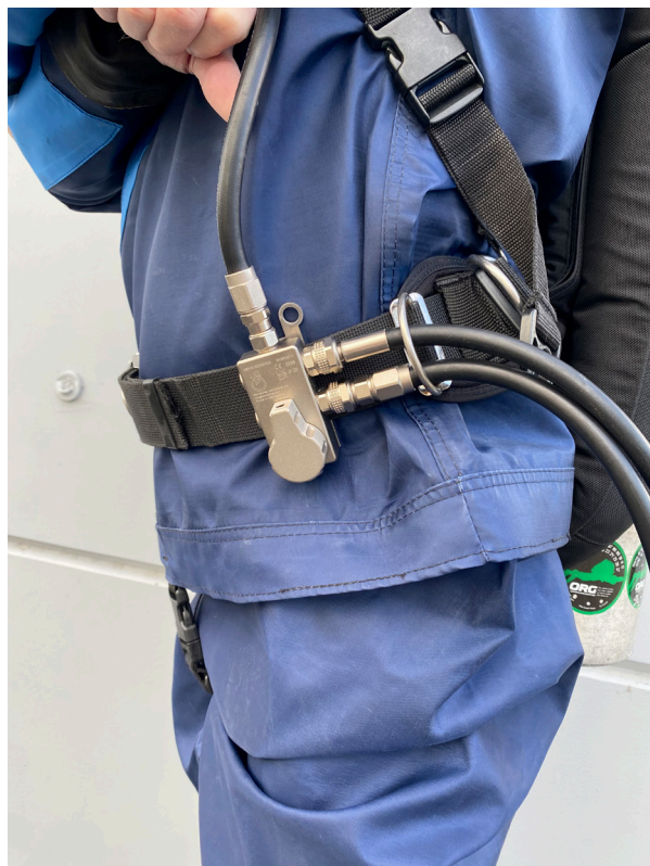
Suggested location for mounting GSB-V2. A 81 cm, (32") low pressure scuba hoses are recommended.
