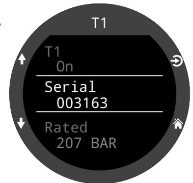
Enter the serial number to pair the transmitter to T1. This number only needs to be entered once. Like all settings, it is stored in permanent memory. Transmitter settings are saved across all dive modes.
