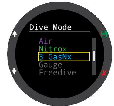
When changing to or from Gauge or Freedive Mode, the decompression tissues are cleared. This is because when in these modes the Tern does not know what gas you are breathing, and therefore cannot track inert gas loading. Plan repetitive dives accordingly.
