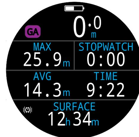
*Standard layout - Alternate Gauge Mode configuration.*
