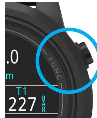
The function (upper right) button is a customizable shortcut that makes accessing your most used functions on the Tern a little easier.
