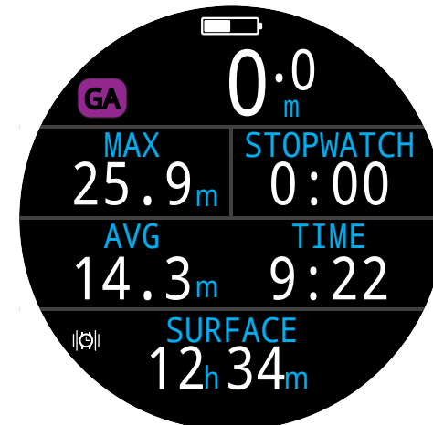
Standard layout - Alternate Gauge Mode configuration.
