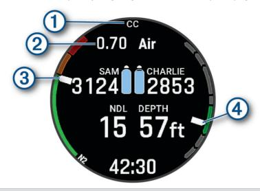
1 Indicates whether closed-circuit (CC) or open-circuit (OC) diving is active.
