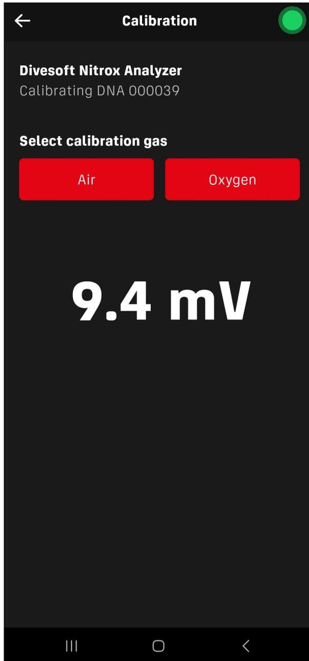
NOTE: Ensure that the sensor voltage value is within the sensor manufacturer's parameters when exposed to the gas. DIVESOFT oxygen sensors have an air voltage range of 7 - 13 mV. It is advisable to verify that the sensor shows linear measurement
