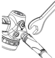
1. If fitted, check the second stage IVS/RVS control switch to ensure that it is set to the "MIN" (-) position prior to connecting your regulator to the cylinder.
