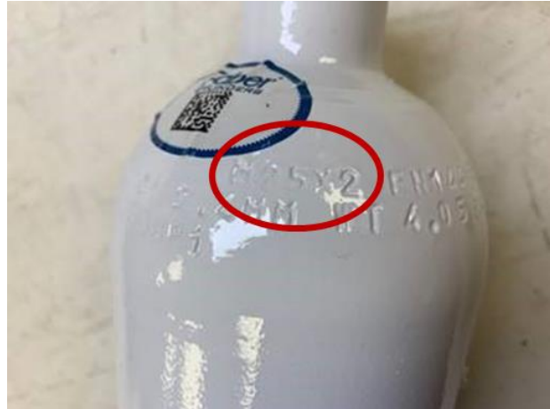
Figure 4 – Example cylinder shoulder stamp marking showing M25 x 2 thread at left side of top row
