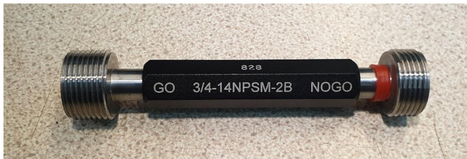
Figure 9 – Example 3/4\" NPSM cylinder plug gauge – Left side GO – Right side NO GO
