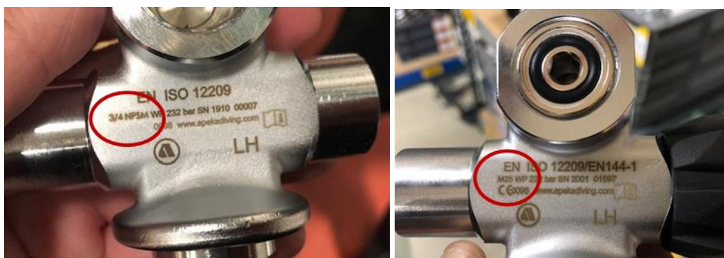
Figure 6 – Example cylinder valves showing 3/4 NPSM (left) and M25 (right) inlet (stem) connection marking
