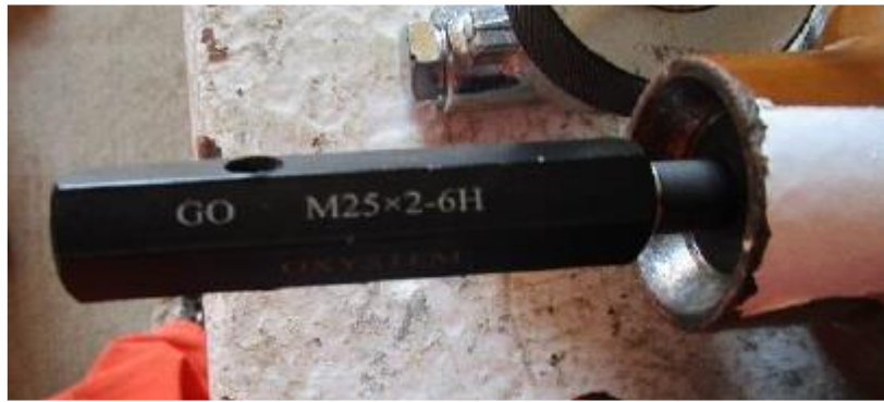
Figure 10 – M25 x2 cylinder plug GO gauge – PASS (fully inserted)
