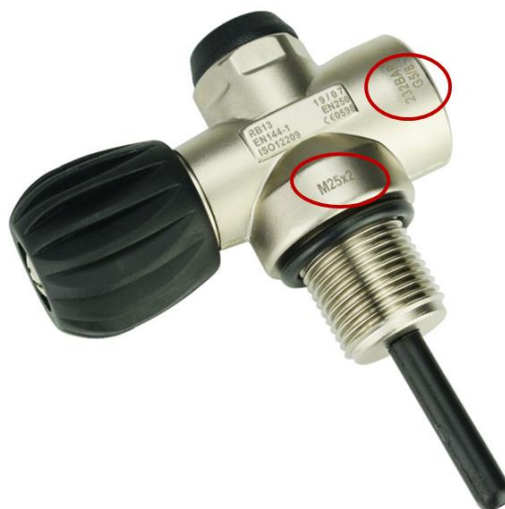
Figure 5 – Example cylinder valve showing marking of M25 x 2 inlet (stem) connection thread and G5/8 outlet connection thread
