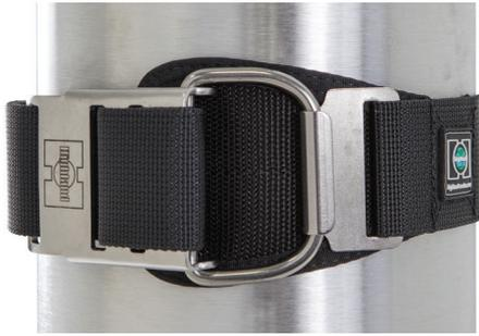
The Highland SS Cam Buckles are not only strong, they provide the added convenience of separating, for quick changeout of your cylinder. Flipping the cam buckle open allows the wire bail to separate from the clasp. There is no need to unthread the buckle. (fig.1)
