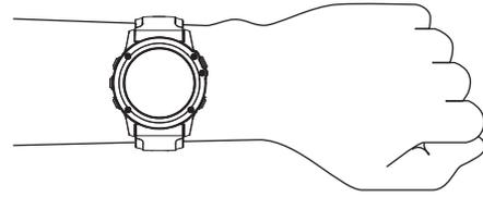
**NOTE:** While diving, the device should stay in contact with your skin, and it should not bump into other wrist-worn devices.
