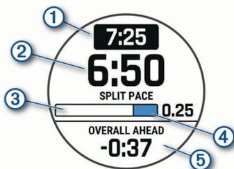
The device displays your target split pace ①, current split pace ②, completion progress for the split ③, distance remaining in the split ④, and overall time ahead or behind of your target pace ⑤.
