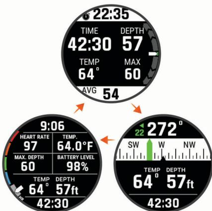
**Dive stopwatch:** Displays the bottom time stopwatch; current, maximum, and average depth; and rate of ascent or descent (*Using the Dive Stopwatch, page 6*).
