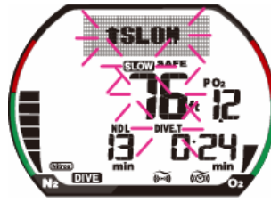
Ascent rate warning with “SLOW” and depth blinking
