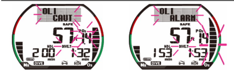
View 1 - OLI warning, "OLI CAUT" and "OLI ALARM" blinking. View 2 - OLI graph also blinking.
